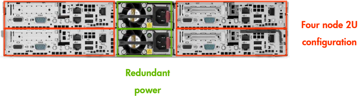
Figure 8. DL1000 four node configuration – rear chassis view
