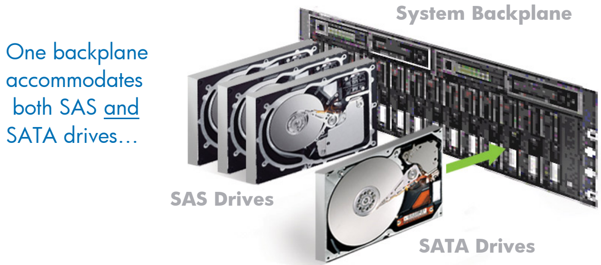
Figure B-3. Common backplane for Serial drives
