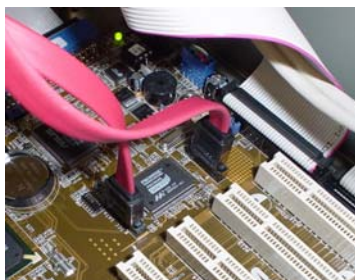
Figure 7. Embedded SATA controller
